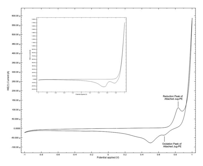
**Fig. 2.** The cyclic voltammogram of attached Jug-PE: A cyclic voltammetry was taken for a 10  $\mu$ M concentration of CP in PBS 0.1 M, containing 2 M NaCl (Potential range: -1.0 to +1.0, scan rate: 0.15 V/s). The obtained data show that the oxidation and reduction peaks for this redox molecule appear in the +0.4 to +0.9 V range of potential axis on the voltammogram. The inset shows the background cyclic voltammetry scan which was taken in PBS 0.1 M containing 2 M NaCl in absence of CP.
