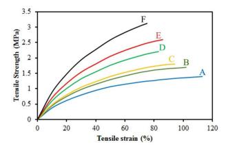
Fig. 3. Tensile evaluation of electrospun mats prepared at collector rotation rates (A) 300 rpm, (B) 400 rpm, (C) 500 rpm, (D) 700 rpm, (E) 800 rpm, and (F) 900 rpm.
