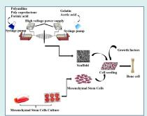
differentiation. Mechanical properties of the fibers were tested. Their hydrophilicity was measured using the sessile drop method. SNL Cells were then seeded onto the fiber, and MTT was performed to assess its toxicity. The cells were then differentiated. After osteogenic differentiation, alkaline phosphatase activity, calcium content assay, and alizarin red staining were done to check the validity of osteogenic differentiation.
