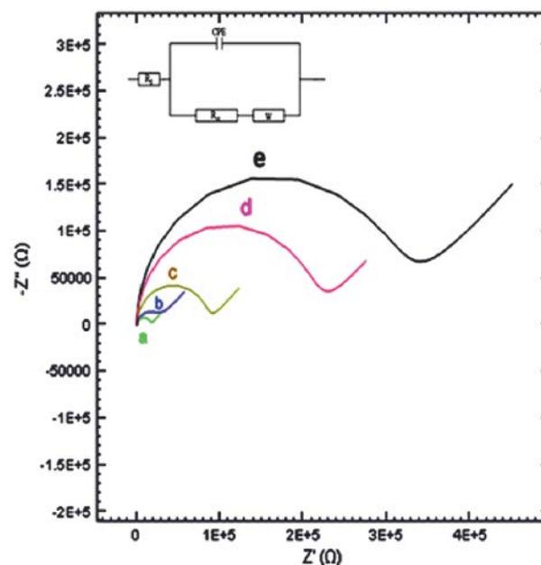
Fig 3. Nyquist plot of different electrodes measured in the presence of 5 mM  $K_3[Fe(CN)_6]/K_4[Fe(CN)_6]$  in Tris buffer 10 mM (pH 7.4) at 25 °C: (a) bare gold electrode; (b) nano-Au modified electrode; (c) unfolded aptaMETH/ nano-Au modified electrode; (d) amphetamine incubated aptaMETH/ nano-Au modified electrode; (e) methamphetamine incubated aptaMETH/ nano-Au modified electrode.
