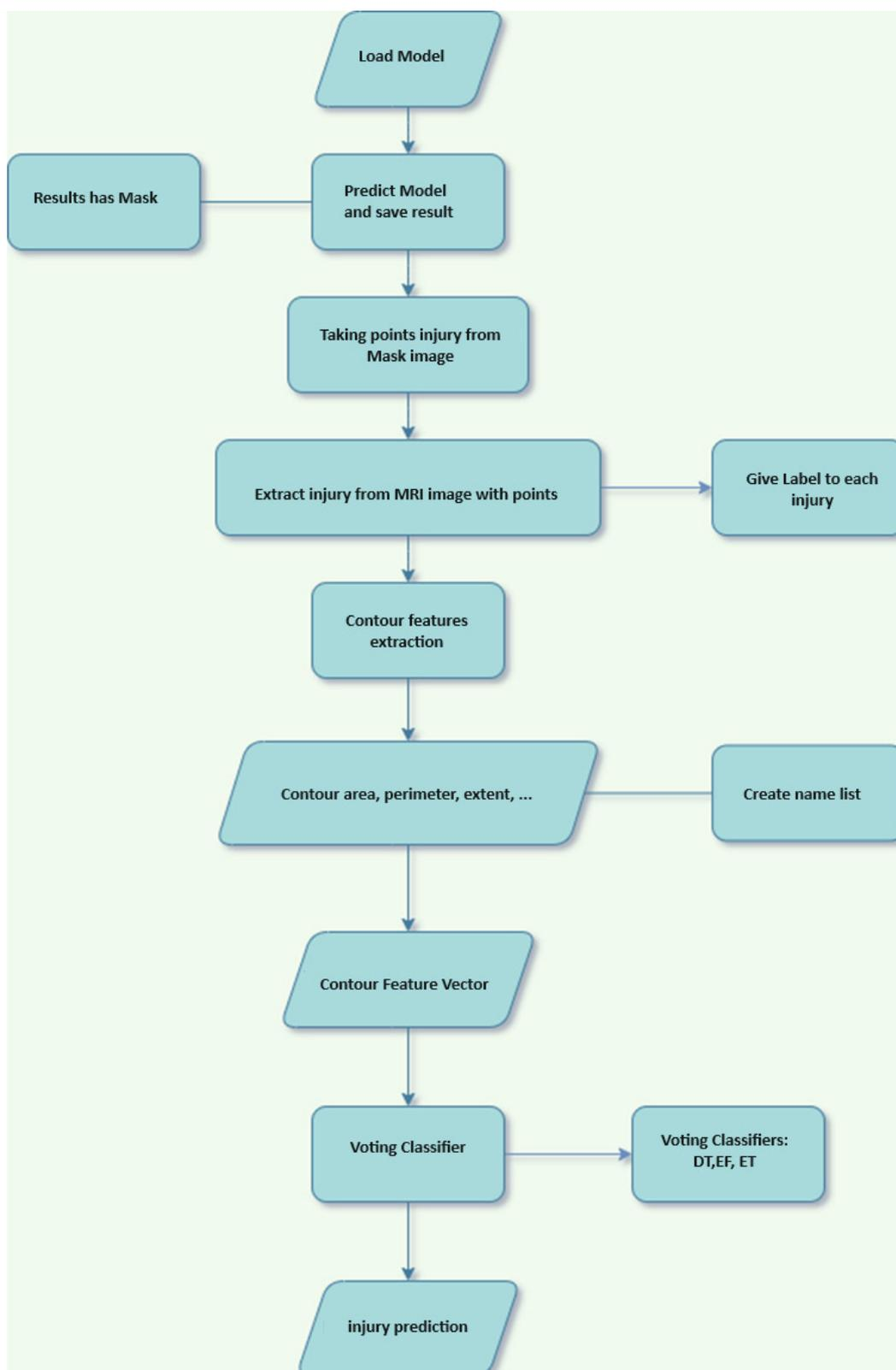
Fig. 4. Flowchart of feature extraction and injury type classification
