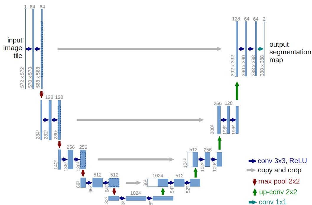
Fig. 2. Typical U-Net neural network architecture.
