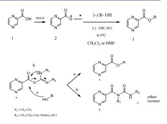
**Scheme 1.** Formation pathways of POE and *N*-acylurea resulted from the reaction of *O*-acylisourea intermediate.
