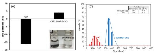
Fig. 4. The Zeta potential of the GO and CMC/MOF-5/GO (A). The stability comparison between GO and CMC/MOF-5/GO (B).
