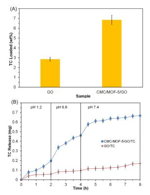
**Fig. 6.** The TC release behavior of GO and CMC/MOF-5/GO bionanocomposite in the conditions simulate to the gastrointestinal tract passage (pH and time).
