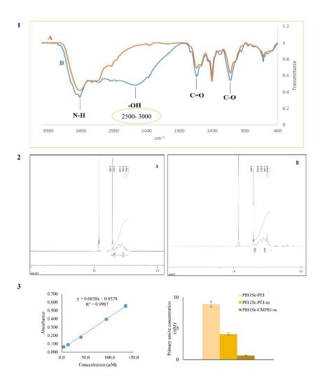
**Figure S1**. FTIR (1) and 1H-NMR (2) spectra of PEG5k-PEI NG (A) and PEG5k-CMPEI NG (B). TNBS assay (3): the calibration curve plotted for the glycine standard solutions in various concentrations (left) and the primary amine concentration in PEG5k-PEI, PEG5k-PEI NG, and PEG5k-CMPEI NG dispersions prepared at similar PEI concentration (0.75 mM).
